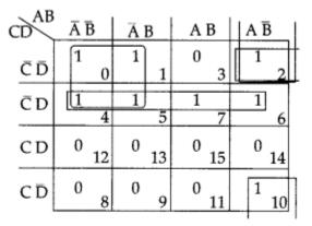
Quad 1 ( $m_0 + m_1 + m_4 + m_5$ ) reduces to Quad 2 ( $m_4 + m_5 + m_6 + m_7$ ) reduces to D Pair 1 ( $m_2 + m_0$ ) reduces to A Hence, F(C, D, A, B) = + D + A
